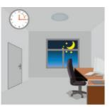
Due to the adjustable twilight value, the luminaire only reacts at night, for example. Off during the day (picture 1) and on at night when you enter the room (picture 2). The adjustable standby function lowers the brightness to 20% when leaving the room for the set time. After the set standby time has elapsed, the light switches off completely.
